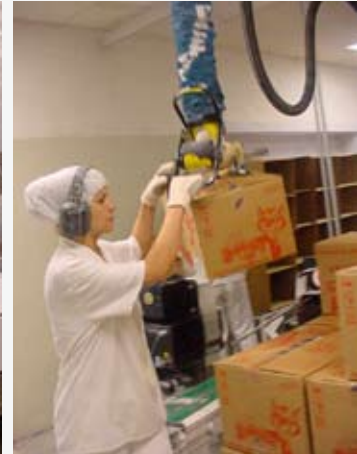
2. Food industry have been using vacuum lifters to handle boxes in the cold packaging area for many years.
