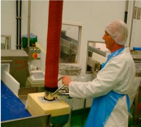
2. This version is a VM120 standard handle with suction foot art nr 630715, stainless steel configuration.
