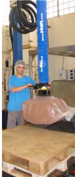
Typical sack lifter installation.
